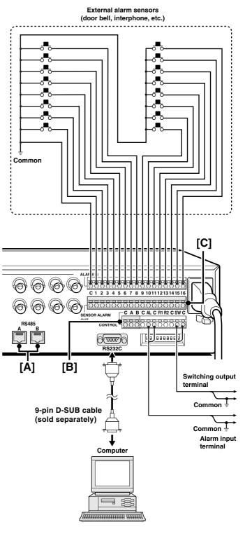
Connect a 9-pin D-SUB cable (sold separately) from the RS232C terminal on the rear panel to the computer serial connector.
